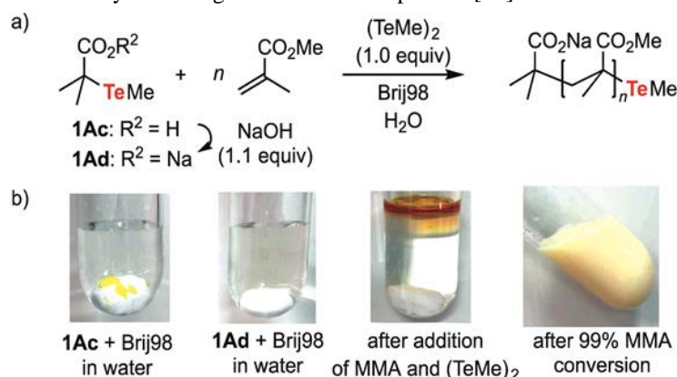
Figure 6. a) Polymerization of MMA by emulsion polymerization and b) solution behavior before and after polymerization *Brij® is a trademark of Croda Americas LLC.
